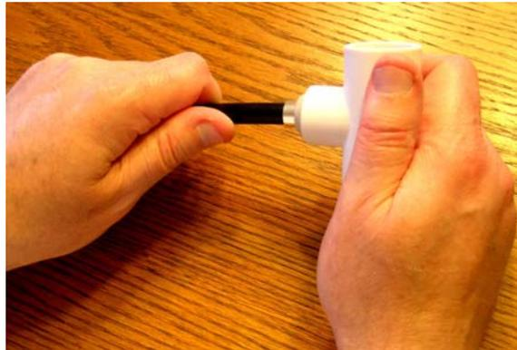
The T-connector side openings allow you to see when the center conductor has reached the tip of the connector. Just unthread the tool from the installed connector and I'm ready to crimp the connector and solder the tip for another flawless installation. For the price of a PVC connector, a leftover PL-259 barrel, and some glue, I have a tool that does the job quickly every time. (Tnx Joe, K9RFZ)
