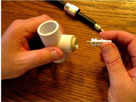
Line up the connector on the coax and twist away.
