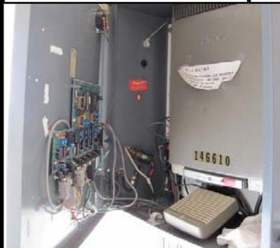
Dave remembers this repeater from back in the 90's, like an old friend. "As I recall, the enclosure came from some old equipment we had retired at work. I gutted out the box and installed an old GE Master 2 the Club had purchased at Tuthill. I spent a couple of Saturday's converting the radio for 2 Meter use and wiring up in this box. The only new thing I see is the controller which has probably changed out several times over the years."
